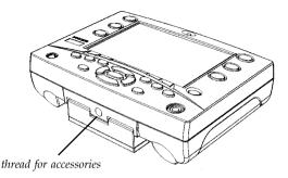
Fig 1.1 - Position of Tripod Mount
