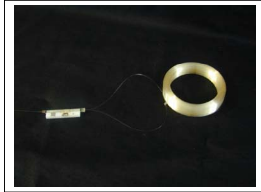
Figure B1 : The “heart” of a FOG the optical fiber coil with its integrated optical circuit
