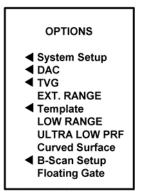
To select a particular item, use the 🛃 and 😭 slewing keys to move the highlight bar up or down the list to the desired item and press **[ITEM SELECT]**. When an item has been selected, the appropriate Set-Up Menu will appear. For example, to review the basic system set-up, the following sequence is used:
