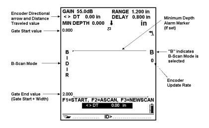
Figure 9.4: Bi-Directional B-Scan Start Screen
