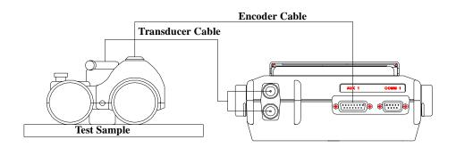
Figure 9.3: Epoch III B-Scan Setup Diagram
