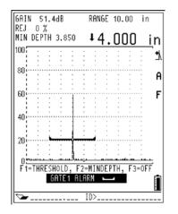
Figure 5-5: Positive Logic Alarm
