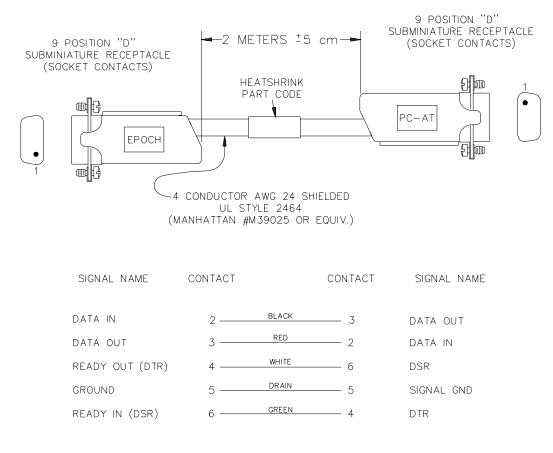
NOTE: THIS CABLE IS REVERSIBLE-THE CONNECTOR TYPE AND FUNCTIONS ARE IDENTICAL.
