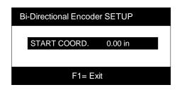
Use the real and real slewing keys to enter the appropriate value for the starting point of your inspection. This will represent the first Distance Traveled (DT) value of the B-Scan. For example, if you are beginning the scan at the end of a pipe or plate, you may wish to enter a value of zero. If beginning a scan a certain distance from the end of the test piece, an appropriate value can be entered.
