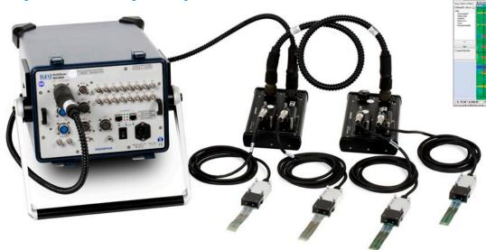
Example of MS5800 with 4x 32-channel ECA probes connected through 2 ECA multiplexers.
