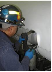
Wet MT is, obviously, messy, and requires surface preparation and post-inspection cleaning before being able to repaint or recoat the weld, which is time consuming. Other shortcomings of this inspection method are its inability to measure the depth of defects and its lack of archiving capabilities.
