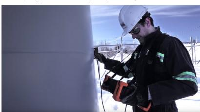
The **Sharck** is also designed to scan at speeds up to 200 mm/s (8 in/s), record inspection data fully, and display it as intuitive 2D/3D C-scans thanks to the **Ectane® 2** and **Magnifi®**. Performing the inspection with the new **Reddy™** (unavailable at the time) could have offered more portability and flexibility.
