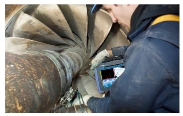
Using ultrasonic techniques, inspection of components can detect cracks, wall loss, and other damage. With the capacity for both angle and linear zero-degree beams, the OmniScan SX is a very cost-efficient solution for this type of single-group inspection.
