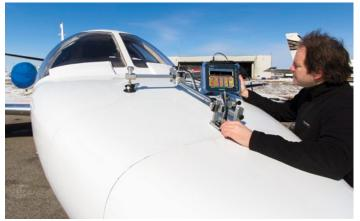
Zero-degree inspection just became even more accessible with the arrival of the OmniScan SX. For corrosion or composite inspection, Olympus offers field-proven solutions for detection of anomalies or wall loss.
