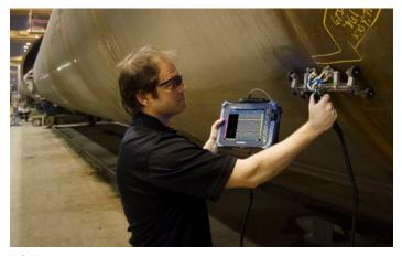
TOFD is an easy and efficient approach for primary detection of weld defects. It is quick, cost-effective and capable of sizing defects present in the volume of the weld, a problematic area for manufacturing defects.
