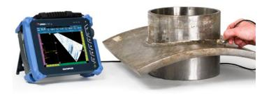
The OmniScan PA is at the heart of the manual and semiautomated phased array weld inspection solutions developed by Olympus for the oil and gas industry. These systems can be used for inspection in compliance with ASME, API, and other code criteria, while offering highspeed detection capabilities, and facilitating indication interpretation.
